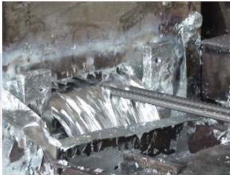
Continuous rebar coating at Xiamen Newsteel, China with Zn-0.2%Al
