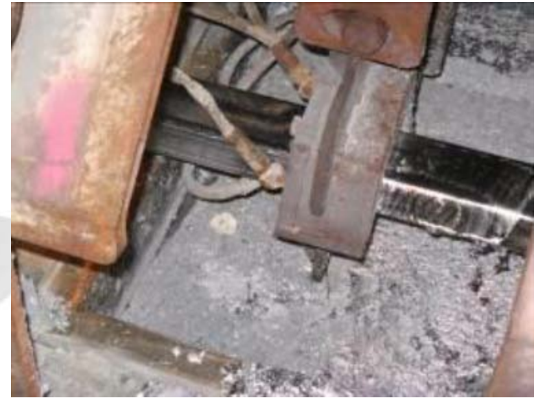
Jet wiping of Zn-12%Al profile at Onesteel, Newcastle, Australia using new dry flux technology
